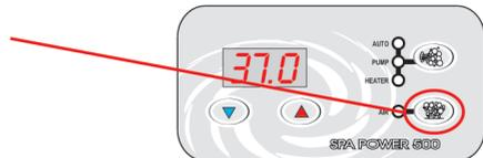
Note: If left on, this accessory will automatically switch off after 20 minutes. If the heater element is on, switching on this accessory may cause the heater to loadshed & switch off. This is to keep the total power load to a safe level.
